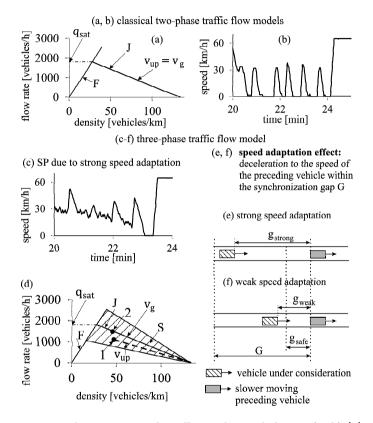
Explanations of oversaturated traffic in classical theory (a, b) [3] and three-phase theory (c–f) [4]: (b, c) Simulations of speed in moving queues (b) and SPs (c). J – line J,  $q_{\rm sat}$  is a saturation flow rate, F – free flow, S – synchronized flow.
